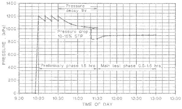
After testing, pipelines shall be depressurised slowly. All air venting facilities shall be open when emptying pipelines. The test water shall be drained to an approved waterway and all connection points shall be reinstated.
