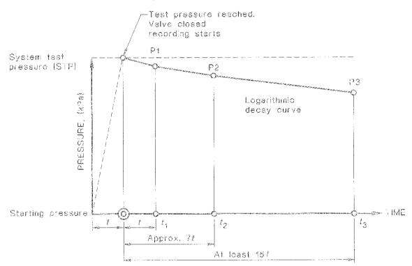
Problems with pipelines may be predicted earlier by comparing the actual pressure with the predicted pressure, which is calculated using the following equation:
